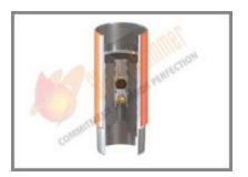
Sledge Hammer's Auto fill float valve permits the casing to fill automatically while being run into the hole. The valve is always in open position, allowing maximum filling of the casing as it running in the well bore. This is especially effective on liner job and sensitive hole conditions. Auto Fill up float shoe can be provided in conventional as well as with non rotating profile.
